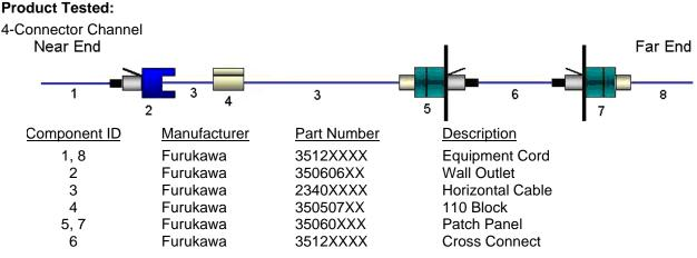
Standard(s)/Specification: ANSI/TIA-568-C.2 Category 6 with the applicable electrical transmission characteristics
